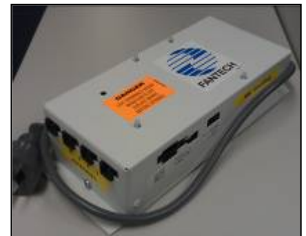
Master Communication Unit
