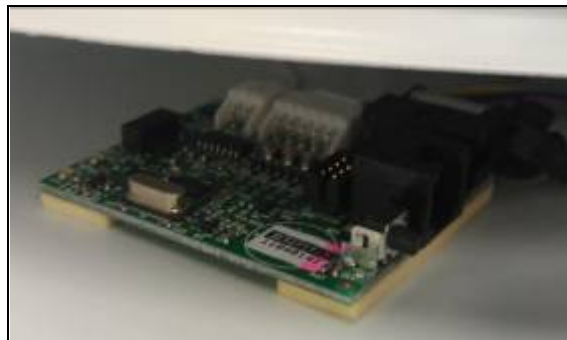
Trim Mounted Control Board
